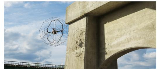
Spherical shell drone for inspecting bridges
